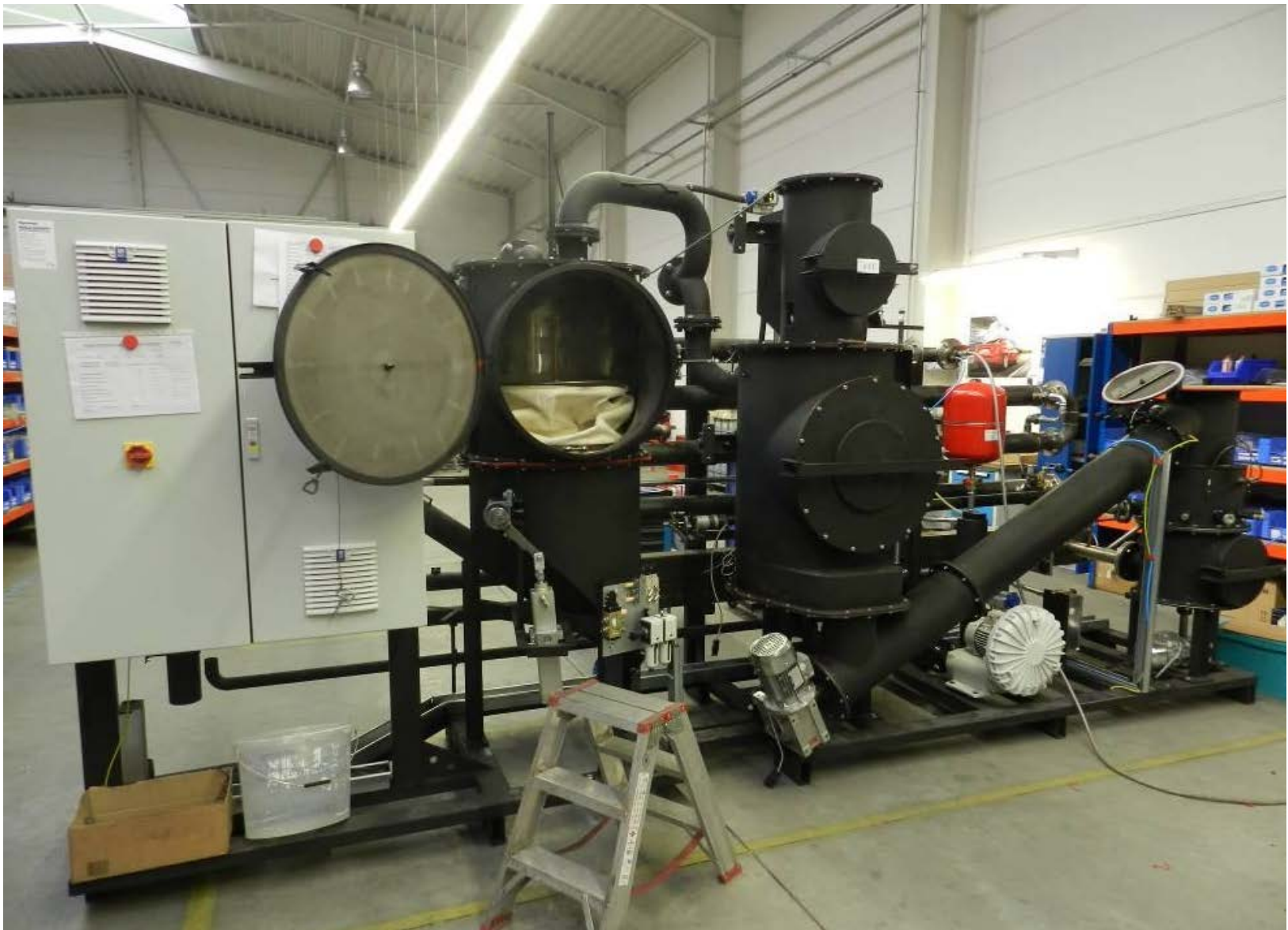
45 kWE SPANNER IN FABRICATION - >300 IN SERVICE 8,000 HRS/YR
