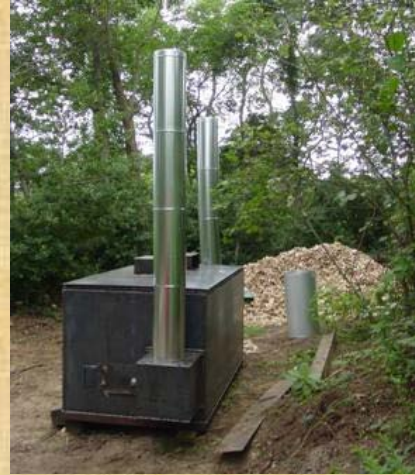
Batch Reactor w/heat recovery newenglandbiochar.org
